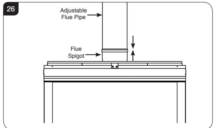
4d.2 Extend the adjustable flue pipe to connect the appliance to the lower mounting plate assembly. The minimum usable length of the adjustable flue pipe section is 300mm, the maximum is 490mm. If necessary use a solid piece of Gazco Balanced Flue pipe to extend the flue connection.
