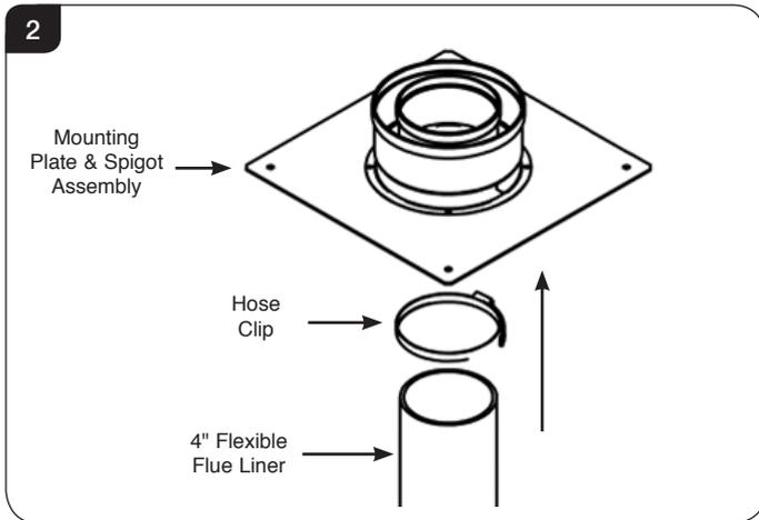
Tighten the Hose Clip so that the liner is held securely to the spigot.
